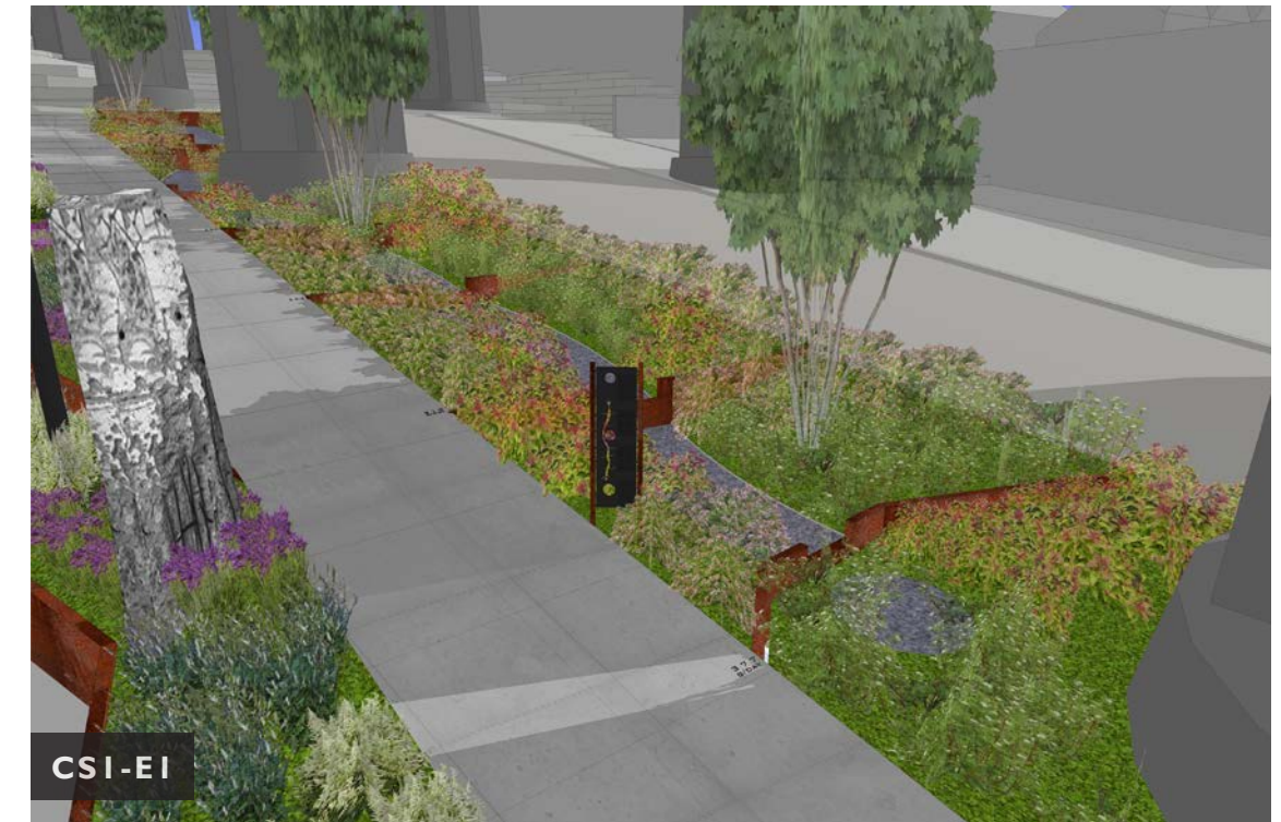
CSI-E1 BIORETENTION TREATING STORMWATER AROUND THE SITE
